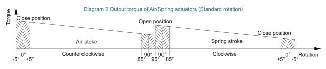
With reference to diagram 2, we can see that the output torque of Air/Spring actuator is not constant but decreasing. This is because of the acting of springs that, when compressed during air stroke, counteract the piston movement and accumulate energy which will be available in a decreasing way during the rotation inversion.
